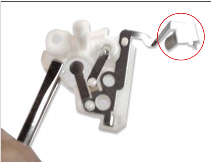
47. Contact plate removed with contoured contact shown intact.
