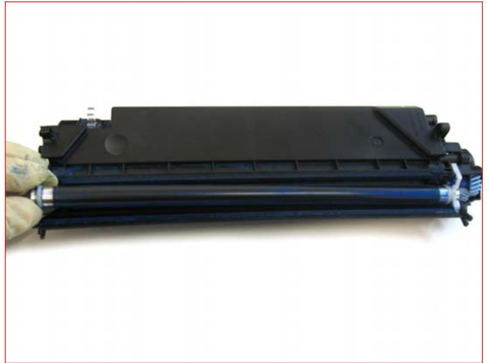
72. Install the developer roller with the gear-side first.
