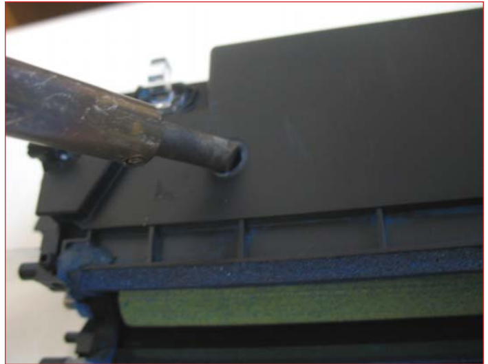
70. Using a soldering tool, create a small hole through the top of the hopper. This will serve as an opening for refilling the cartridge.
