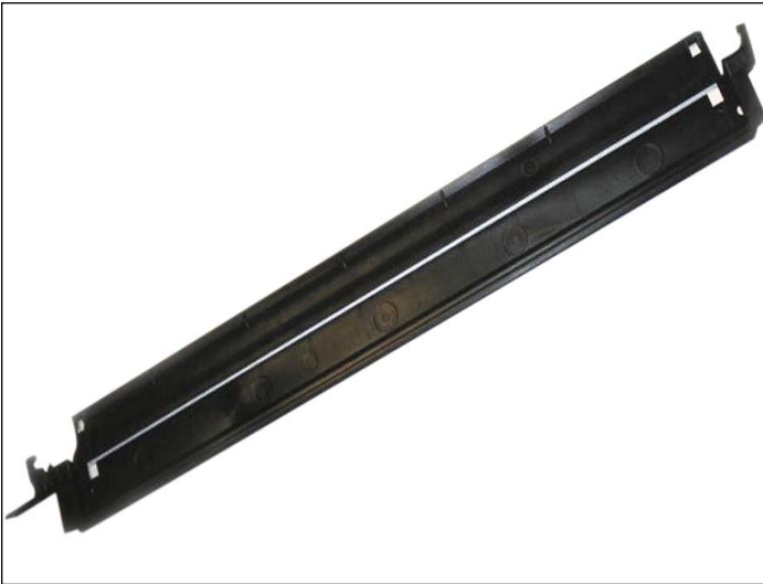
15. Drum shutter completely removed.
