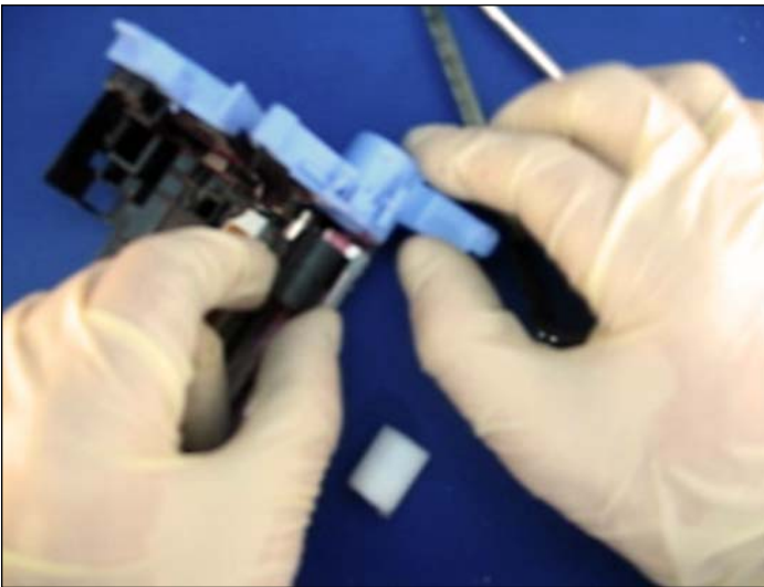
40. First, lubricate the blue axle housings with a minimum amount of white bearing grease. Insert the new non-contact spindle into the housing as shown.
