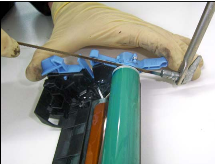
17. Using a hacksaw, cut halfway through the spindle.
