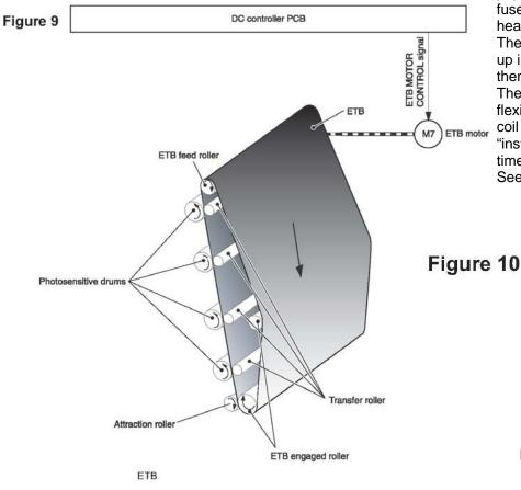
drum and the ETB. As the ETB passes the transfer charging roller, the positive charge is picked up, and draws the negatively charged toner off the drum onto the paper. This process is repeated for each color cartridge. As the toner piles onto the paper, the positive charge on the paper weakens as the paper runs through each cartridge. For this reason, the charge is increased on the transfer charging roller for each successive color.
