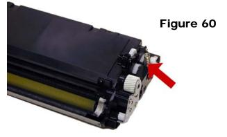
34) Vacuum the feed roller clean. Until new felt seals are available for the developer roller, we do not recommend that the feed rollers be removed. Re-using old seals that have been removed may cause leaks See **Figure 61**
