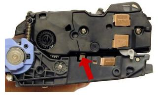
46) Replace the chip on the cartridge. Be sure to use the correct color chip for your cartridge. See **Figure 81**
