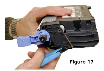
2) Unhook the spring from the bottom left of the contact side of the cartridge. The top half will stay under the blue handle. See **Figure 18**
