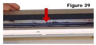
18) Lubricate the new wiper blade with your preferred lubricant. Install the blade and 2 screws. Make sure the wiper blade seal (which ever type you are using) seals along the back edge of the blade. See **Figure 40**
