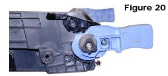
5) Remove the spring loaded drum cover arm. Do not lose the spring! See **Figures 21 & 22**
