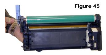
23) Align the drum hub and axle so that the holes line up. Insert the larger of the two metal pins and tap into place with the pin punch. Make sure the pin is centered on the axle. See **Figure 46**
