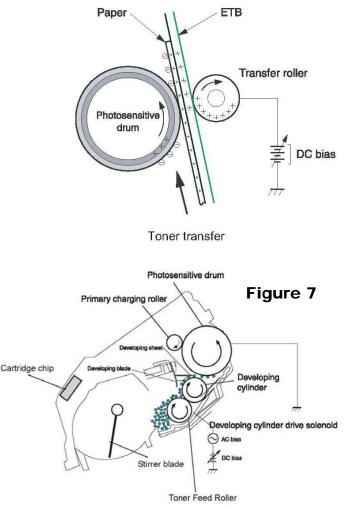
The fifth stage is the transfer stage. This is where there are some large differences from monochrome printers. The first step in the transfer stage is where the attraction roller places a positive DC bias which charges the paper positively to make the negatively charged toner easier to transfer onto the paper during the transfer operation. See Figures 8 & 9
