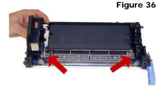
16) These cartridges have a simple auger/plate system that moves the waste toner from behind the wiper blade
