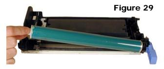
10) On the PCR, note the coating of conductive grease on both sides of the roller. Normally this is only on one side. For these cartridges it needs to be on both. See Figure 30.
