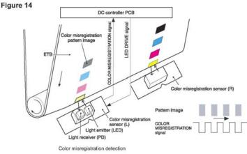
There is also what HP calls the color "misregistration" detection. This is where pattern images are printed to the AETB and detected by various sensors. This is done to correct for any registration problems that may be occurring. See Figure 15
