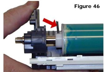
24) Install the metal bearing, drive gear and pin onto the drum axle. Tap the pin into place with the pin punch. Using a small block of wood as a brace under the drive gear will make installing the pin easier. See **Figures 47 & 48**
