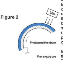
In the first stage, Pre-Exposure LED turns on and wipes any residual charges from the drum surface. This brings the drum surface potential to 0 (zero) volts and helps prevent back grounding. See Fig. 2
