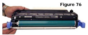
44) Set the two shipping locks on each side of the cartridge. The shipping locks are built in on these cartridges. When the cartridge is installed, the locks will open. Make sure you reset them after the cartridge has been tested. The shipping locks help keep the developer roller from getting a flat spot, which will cause horizontal voids in the print. See **Figures 77 & 78**
