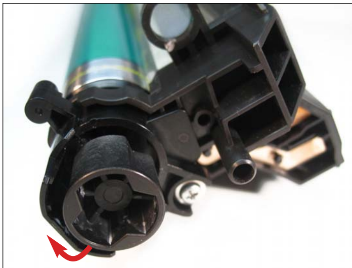
46. Rotate the support clockwise until it locks into place. Once it locks it will need to be secured with its appropriate screw.
