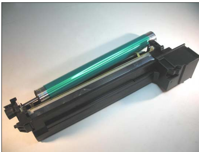
44. Before inserting the OPC, make sure its gears are facing in the correct position.
