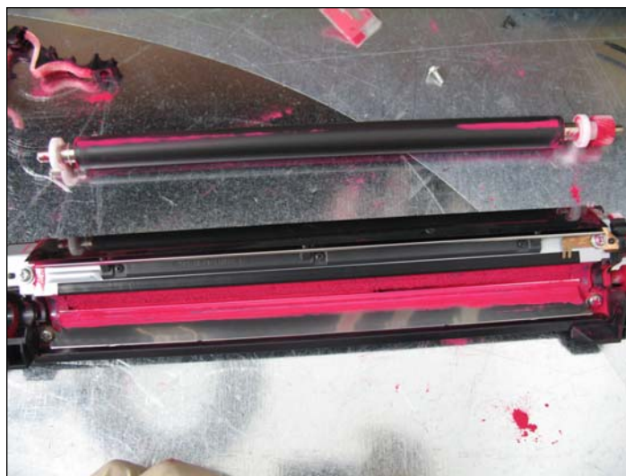
19. DVR roller removed. Remove the two screws that hold the doctor blade.
