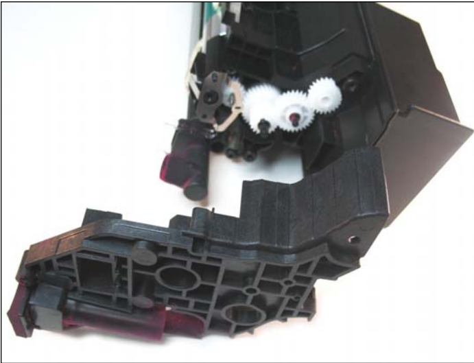
56. Once the chip has been installed, you can proceed with installing the inner section of the end cap.
