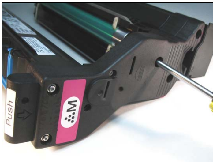
59. Secure the end cap with the seven screws.
