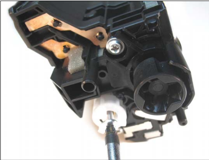
49. Install the developer roller drive gear and its appropriate screw.
