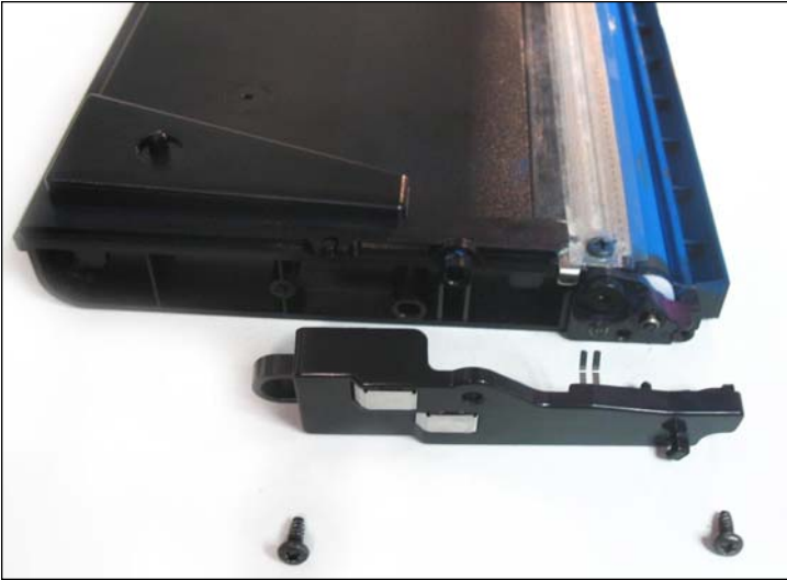
9. End plate removed.
