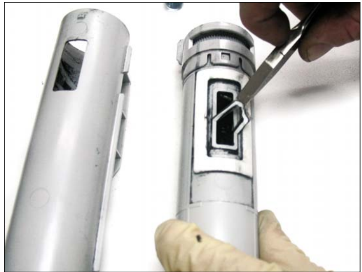
10. First, using a pair of pliers, gently peel off the worn sealant (shown) from the toner cartridge.
