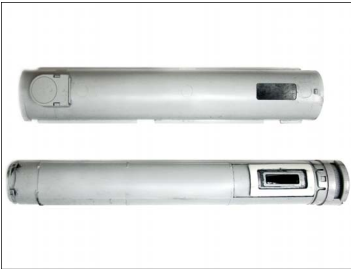
9. Cartridge separated. Note the original positioning of the outer container. Clean thoroughly using compressed air.
