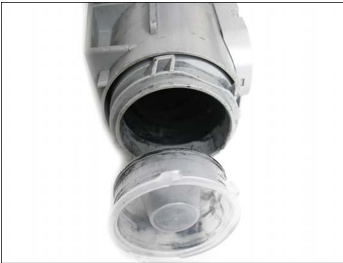
7. Toner fill plug removed. Note the original positioning of the plug for reassembly.
