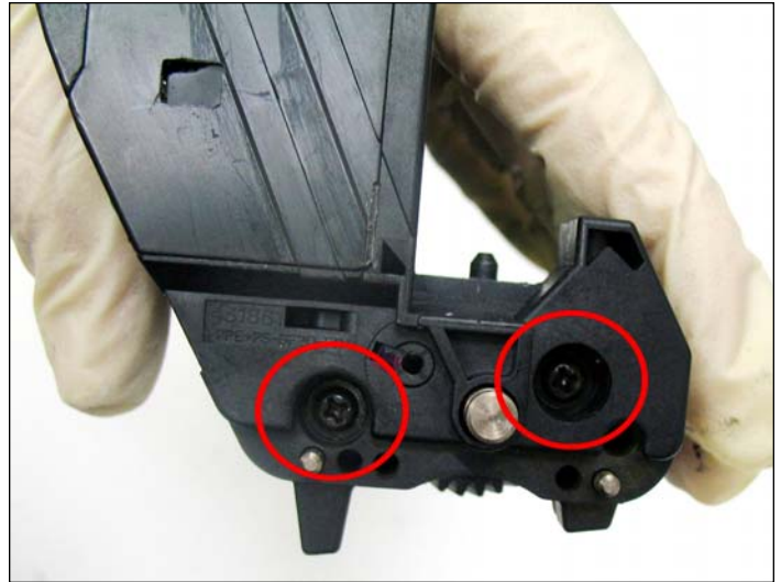
21. Once the drum axle has been released from the opposite side, remove the smaller end cap by removing the two screws shown.
