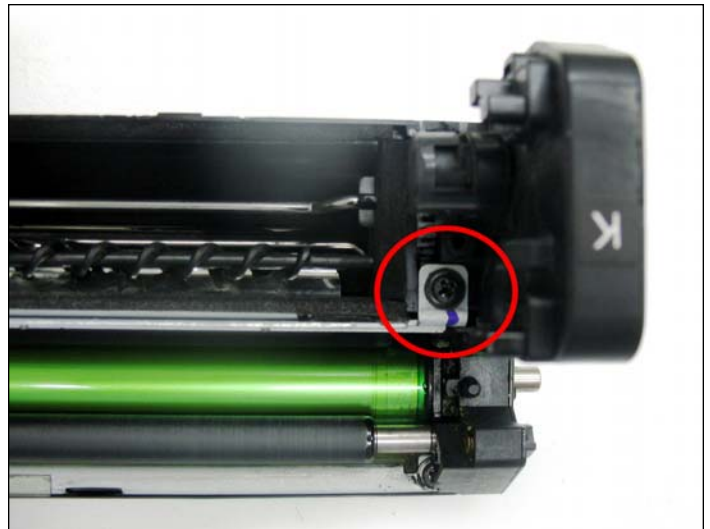
15. Remove the doctor blade by first removing the two screws that hold it in place.
