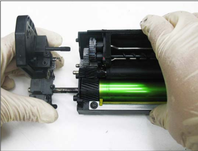
22. Once the drum axle has been released from the opposite side, remove the smaller end cap by removing the two screws shown Pull out the smaller end cap.
