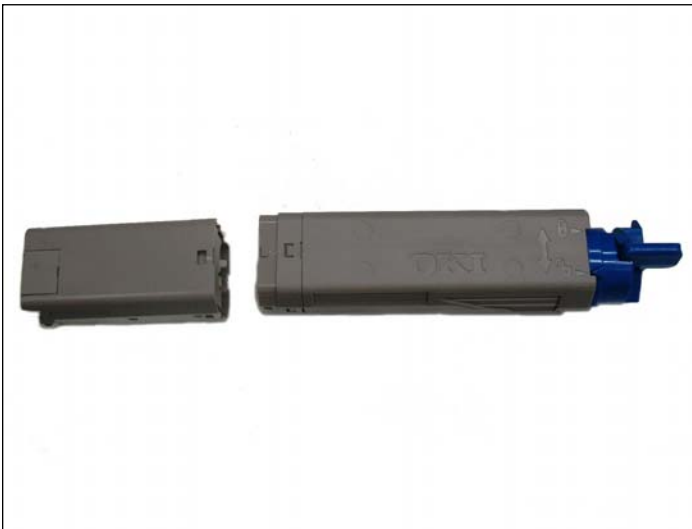
6. Waste section removed.
