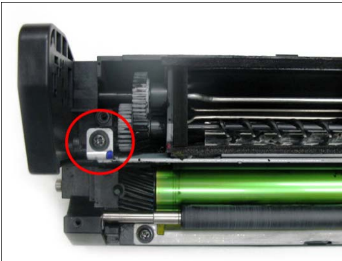
15. Remove the doctor blade by first removing the two screws that hold it in place.
