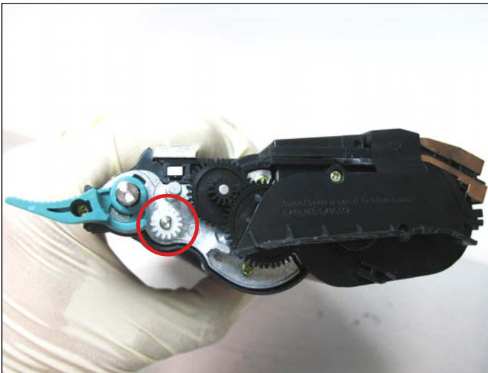
NOTE: Please use extreme caution when removing the supply roller gear (circled) as it is very fragile and might break if removed forcefully.
