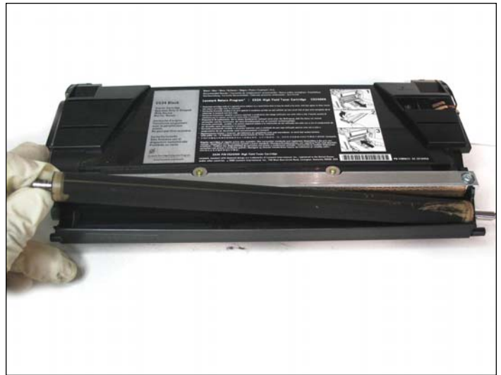
12. Remove the DVR roller.
