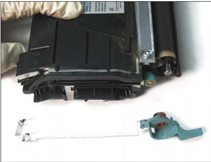
11. Once the DVR support plate has been released, removed with the rear contact as shown.
