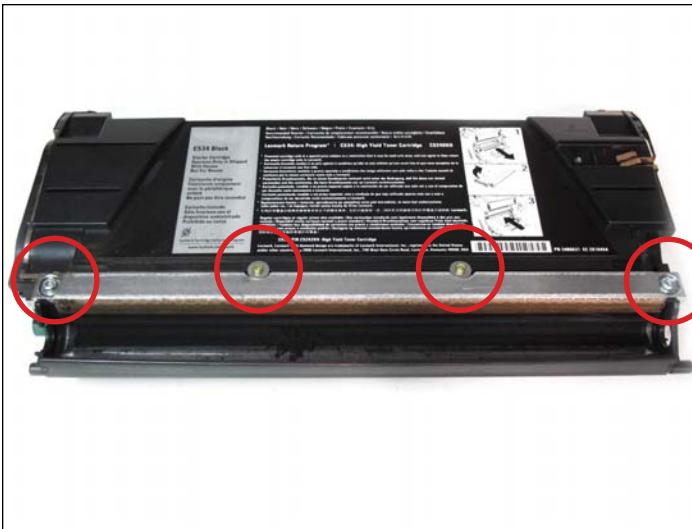
13. Remove the doctor blade by removing the four screws as shown. Note: the location of the doctor bar. It needs to be positioned in the same manner as before.
