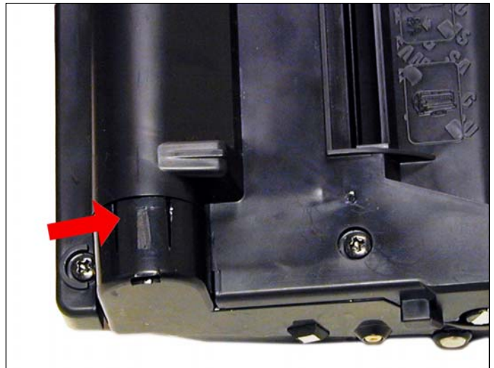
25. Install the remaining end cap and two screws. Make sure the top of then end cap snaps into place over the fill plug
