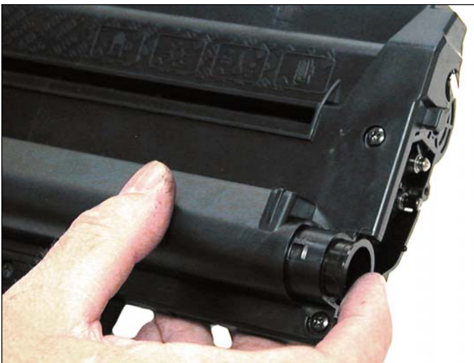
24. Install the fill plug, check for leaks.
