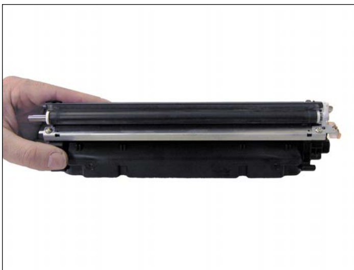
20. Install the developer roller.
