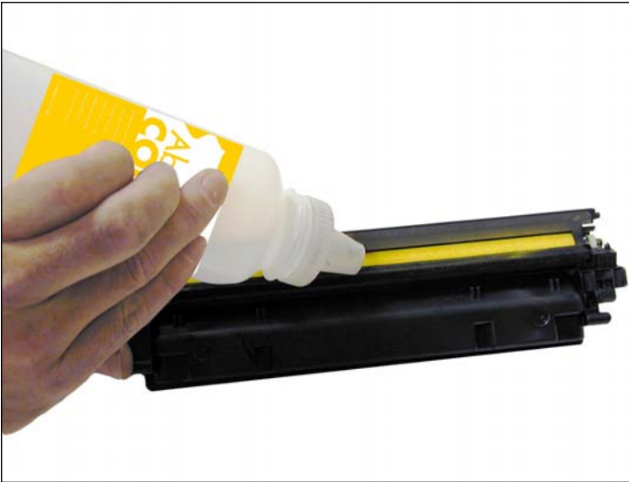
14. At this point, while tight, you can clean and fill the hopper with 2025 toner.
