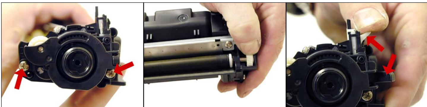
22. Install the gear end cap and screws. Turn the developer roller so it mates properly with the drive gear. Make sure the spring arm works!
