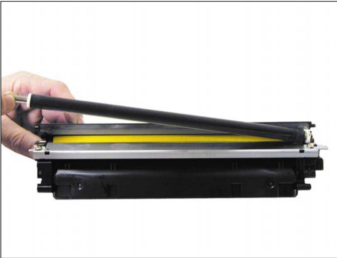
12. Slide the developer roller over and remove.
