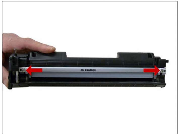
17. Remove the doctor blade and two screws.
