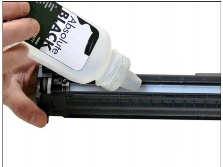
19. Fill through the Mag roller opening with 110g of P2035 toner for the "A" cartridge, 290g for the "X". There is not a fill plug in these cartridges.
