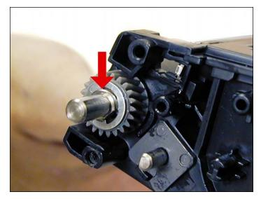
17. Install the developer roller gear and E-ring.
