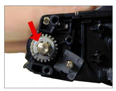
7. Remove the E-ring and developer roller gear.
