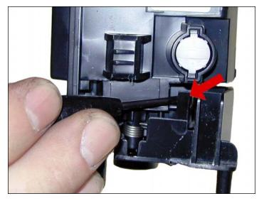
5. Lift up on the tab indicated and remove the end cap.
