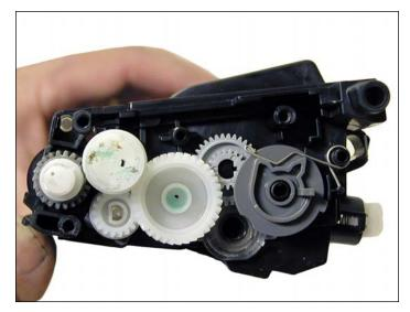
6. Remove all the gears and reset spring.
