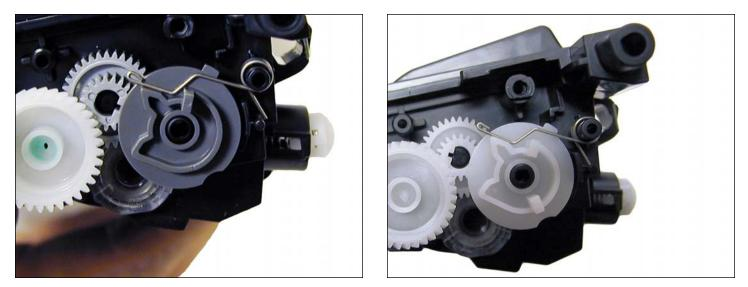
19. Set the reset gear and spring as shown. The tail of the spring fits into a notch at the base of the gear. There are different gears for the TN-110 and TN-115. Each should be set as shown.
