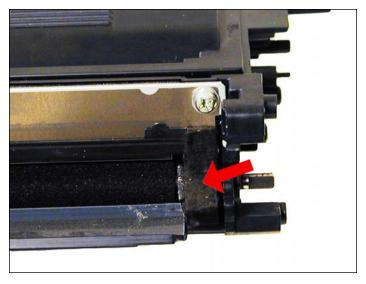
12. Vacuum/blow the doctor blade. We do not recommend that the doctor blade be removed as the developer roller felt seals will be disturbed. Once a new blade is available, great care will have to be taken not to tear the seals causing a leak. The doctor blade can be easily cleaned by blowing the excess toner off, and wiping down with a lint free cloth. Be very careful not to leave any lint behind and do not use any chemicals to clean it!
