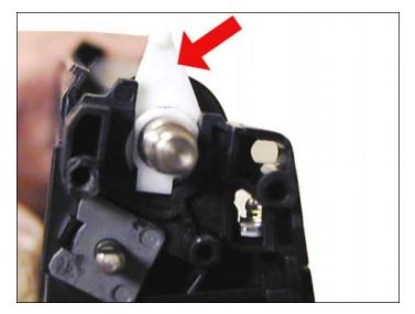
8. Move the white plastic locking tab on the right side of the developer roller to the up position.
