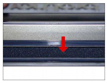
11. Vacuum/blow the cartridge clean. Be sure to rotate the foam feed roller so it is fully cleaned.
