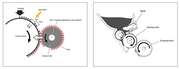
As the laser exposed areas of the OPC Drum approach the developer roller, the toner particles are attracted to the drum's surface due to the opposite voltage potentials of the toner, and laser exposed areas of the OPC drum.
