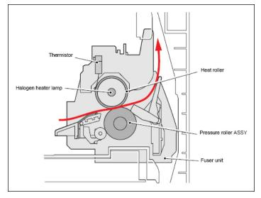
In the **fifth stage**, the image is then fused onto the paper by the fuser assembly. The fuser Assembly is comprised of the upper heating roller and lower pressure roller. The lower pressure roller presses the page up into the upper heating roller which then melts the toner into the paper. This heating assembly consists of a hard metal coated roller with a halogen lamp inside.
