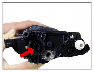
2. Remove the fill plug from the toner cartridge. Dump the remaining toner and vacuum/blow out the cartridge. There will probably be a label over the fill plug. It comes off with a little alcohol and a lint free cloth or cotton swab.
