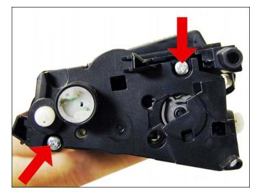
4. With the handle facing you, remove the 2 screws on the left end cap.
