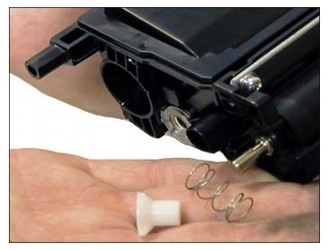
9. Gently pry off the white bushing on the opposite side of the developer roller. Be careful not to lose the spring!
