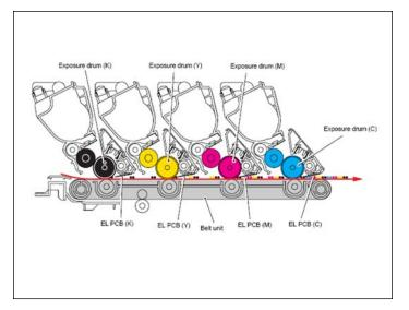
The **fourth stage** is the transfer stage. In the transfer stage the transfer roller which is located directly opposite each OPC drum, places a positive DC bias charge on the back of the Image Transfer Belt. Each toner cartridge has a separate transfer charge roller. The image is transferred from the drum directly to the paper. This process is repeated for each color cartridge in the following order: Black, Yellow, magenta, and cyan.
