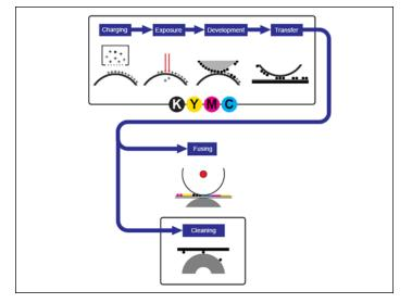
This simple diagram shows the 6 basic steps in the printing process.
