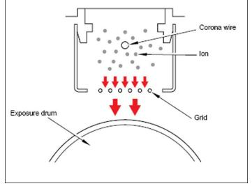
In the **first stage**, the Primary Corona Wire places a uniform 870VDC voltage on the Corona wire grid which then charges the OPC drum surface. The amount of the DC voltage placed on the drum is controlled by the printer's intensity setting.
