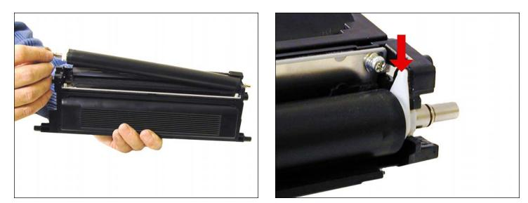
15. Re-install the developer roller long shaft side to the gear side, and white lock pointing up. Turn the lock towards the doctor blade until it locks in place.
