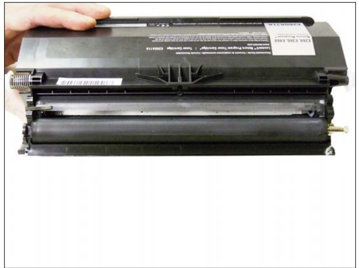
14. Wipe the developer roller with a clean lint free cloth, and re-install the developer roller. At this point we do not recommend that any chemicals be used to clean this roller. Install the keyed end of the roller to the gear side.
