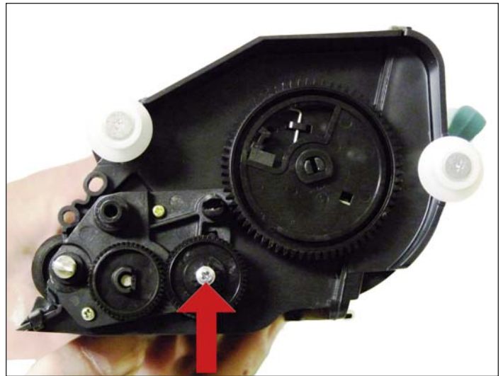
9. Remove the screw and lower idler gear.
